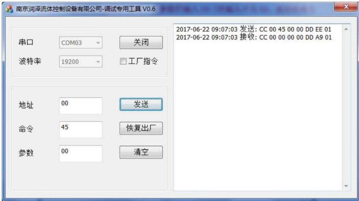
3. Use command 44, input 00 in the address bar (if the address is changed, input the changed address), input 44 in the command bar (The motor rotates through the code disc, and the optimal path is automatically selected), input 04 in the parameter bar and click to send. The switching valve will rotate to port 4 which is connected to the common port now. The received command after turning to the port 4 is as shown in Figure 4-6
