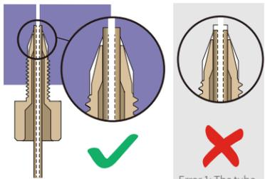
Note: Make sure the tube is properly installed to the bottom of the port, introducing dead volume
