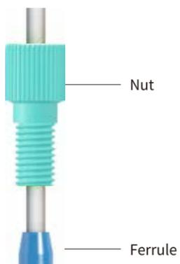
✘ Make sure the ferrule is oriented correctly! The narrow end of the ferrule should towards the nut.
