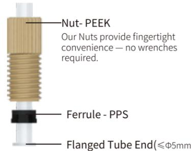
※ Make sure the ferrule is oriented correctly! The narrow end of the ferrule should towards the nut.
