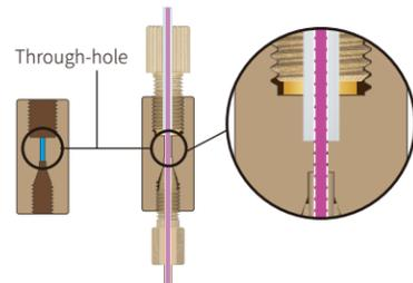
※ The wetted liquid volume is shown in the figure for the volume of the threaded port connection channel
