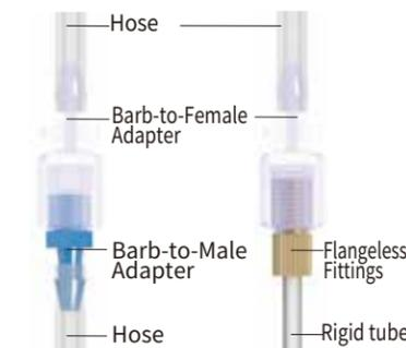
※ Can be used with RUNZE flangeless fitting, flanged fitting and barb-to-male adapter to allow for any connection between rigid tube and rigid tube, rigid tube and hose, hose and hose of the same or different tube diameters
