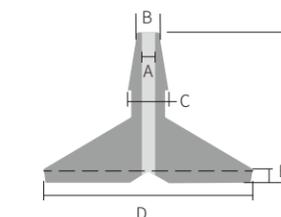
The bottom of the barbed sink head is designed with a 120° groove, which enables the liquid to flow out stably in time while maintaining its own stability.
