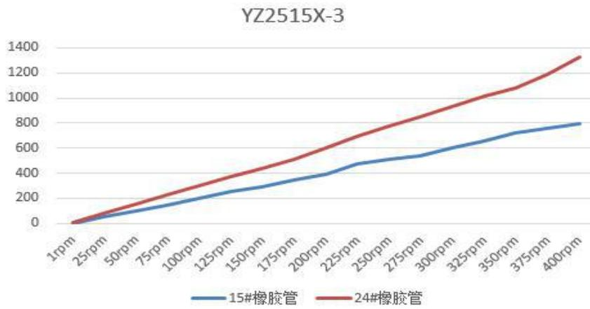
Figure 6-2-3 YZ2515X-3 rollers (LM60A) flow-speed curve
