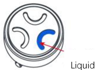
Figure 2-5-2 Dead volume (Sealed rotor)
